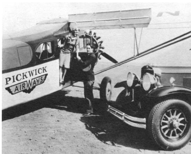
Trailing edge of wing folded forward to allow passenger entrance into cabin of the Fairchild 71. (Herman Rubin)
