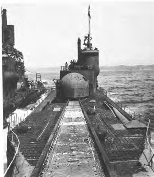
Imperial Japanese Navy's I-14 at Sagami Bay after surrender. Retractable crane on port side. (U. S. Navy)
