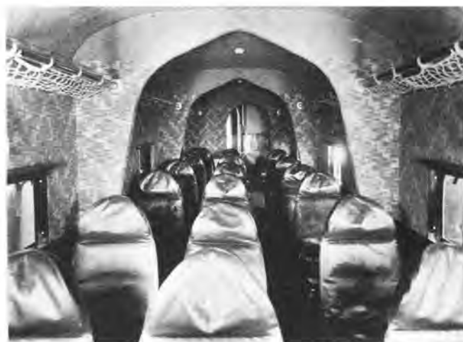
Fifteen-passenger day seating arrangement in YC-30 Condor, probably C/N 26. (USAF Photo 18572 AC)
