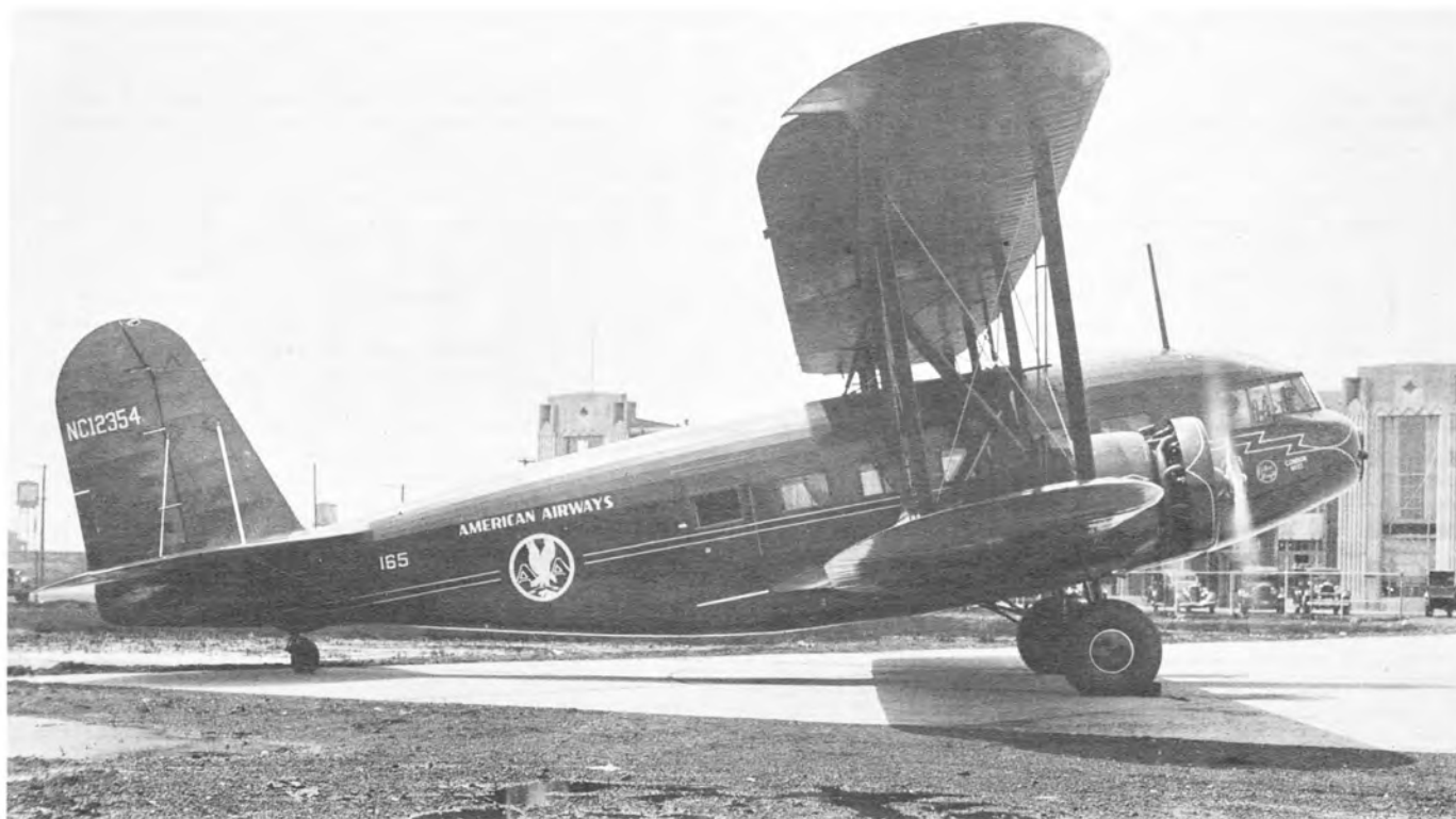
Difference between early and late Condors can be seen in these two photos. Above is the second T-32, C/N 22, at Newark while below is the first Condor built new to have increased gross weight of 17,500 pounds, AT-32A, C/N 42. American Airlines name change and slight trim differences can be seen. (John C. Barbery & Merle Olmsted)
