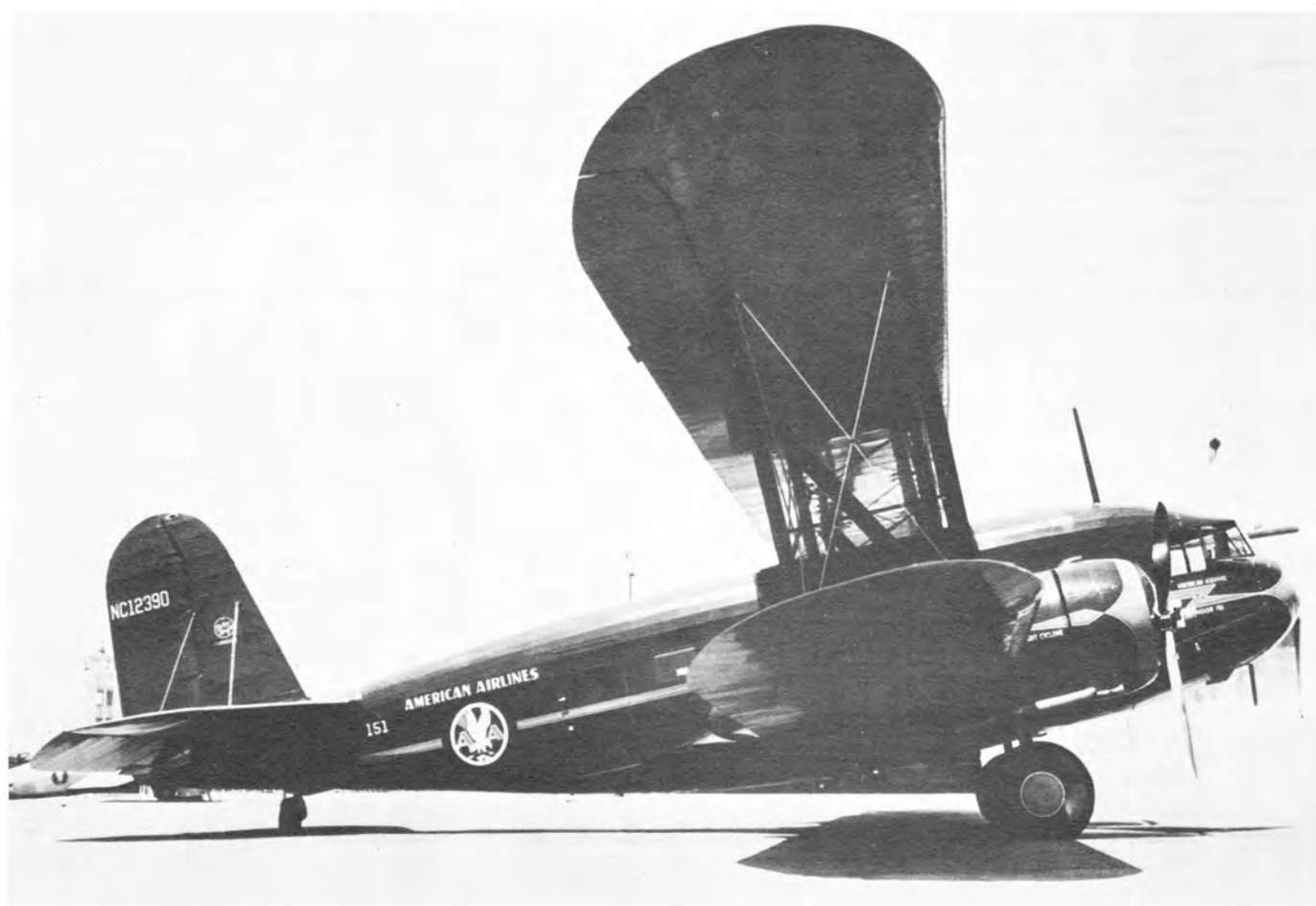
Difference between early and late Condors can be seen in these two photos. Above is the second T-32, C/N 22, at Newark while below is the first Condor built new to have increased gross weight of 17,500 pounds, AT-32A, C/N 42. American Airlines name change and slight trim differences can be seen. (John C. Barbery & Merle Olmsted)
