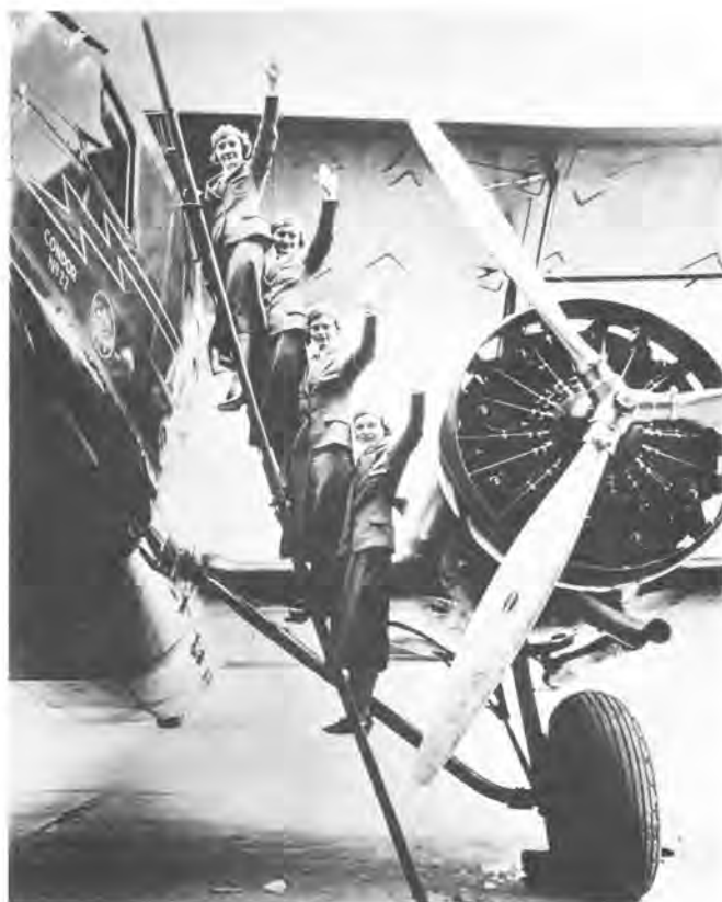
Publicity photo of C-124, and contemporary beauties, showing fixed pitch propellers, some of the many access panels, and the recess for the undercarriage radius rod when retracted. (American Airlines)
