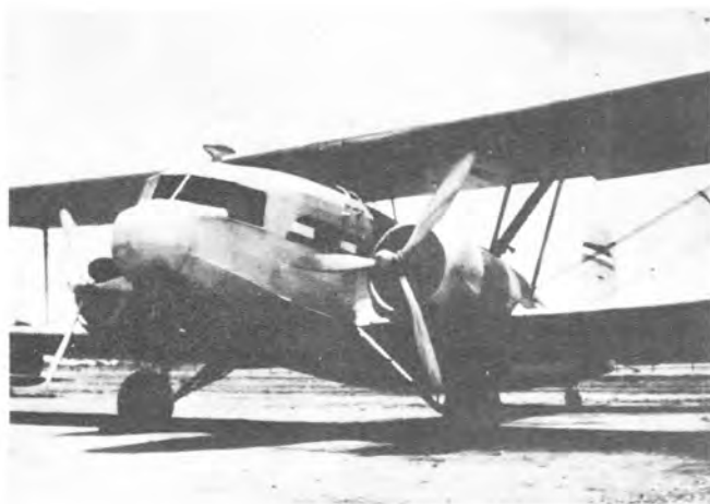
C/N 21 in 1947, registered XB-GIT, with AT-32 type cowlings and constant speed propellers. Fuselage stripes probably red-white-green. (Jose T. Villela, Jr.)
