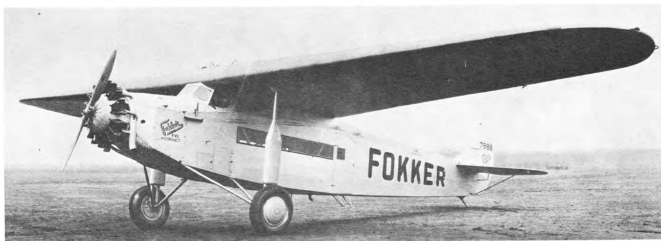
The last American F-VII delivered, C/N 617 with registration 7888 (later NC-7888). Fitted with 525 hp P & W Hornet engine and used by Standard and Universal Airlines on the Los Angeles to El Paso run. (American Fokker)
