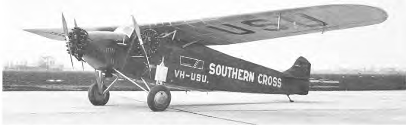
The SOUTHERN CROSS after rebuild at the Dutch Fokker plant during its westward voyage of 1930. Wing now painted silver. Note concession made by Australian government in waiving size and location requirements for fuselage registration letters to permit the retention of the now famous name of the airplane. Lettering FOKKER F-VIIB/3M appears on the rudder. (Netherlands Fokker Photo)
