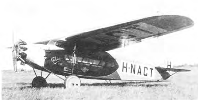
Single engine Dutch Fokker F-VIIA with Bristol Jupiter engine. Coloring and most markings are identical with the prototype Trimotor which was hurriedly converted and brought to the U. S. for the Ford Tour. (Fokker)
