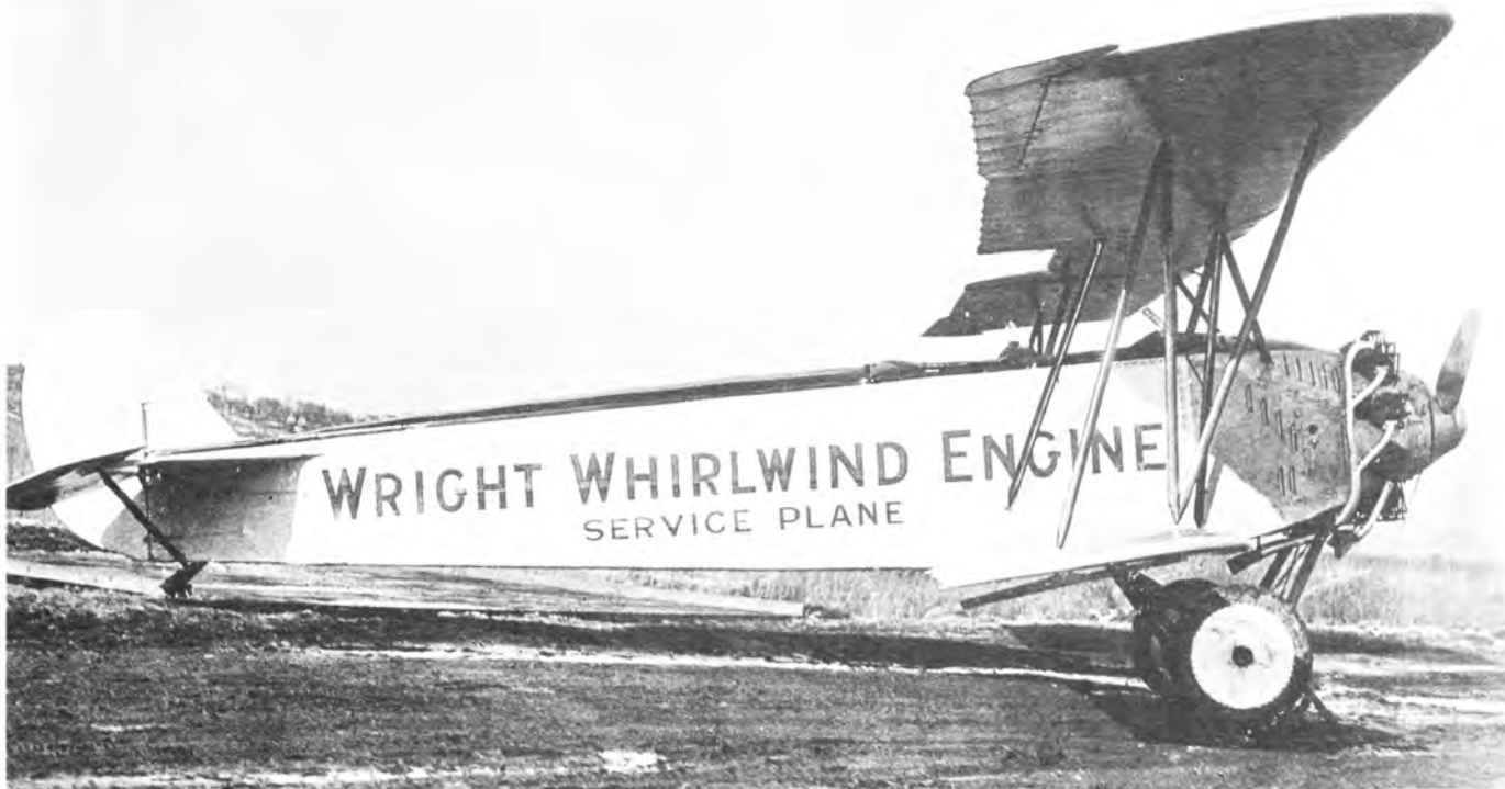
Modified form of S-3 with 200 hp Wright J-4 radial engine. Compare wing with similar view of Hiss-powered model: enlarged cutout, slight sweepback and ailerons projecting behind the trailing edge. (USAF Photo 33536 AC)
