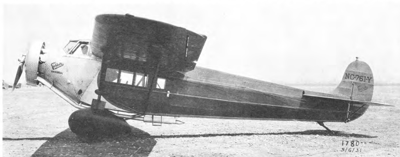
Deluxe Wright J-6 powered Universal with enclosed pilot cabin, Townend drag ring and wheel pants. Photographed at Teterboro on May 6, 1931, aircraft is C/N 439. (American Fokker Photo 1780 from North American Aviation)
