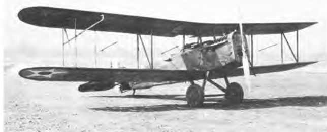
The XC0-8, a DH-4M2 fitted with Loening COA-1 wings, retaining its original wood undercarriage but fitted with early adjustable steel prop. (McCook Field Photo 24257)
