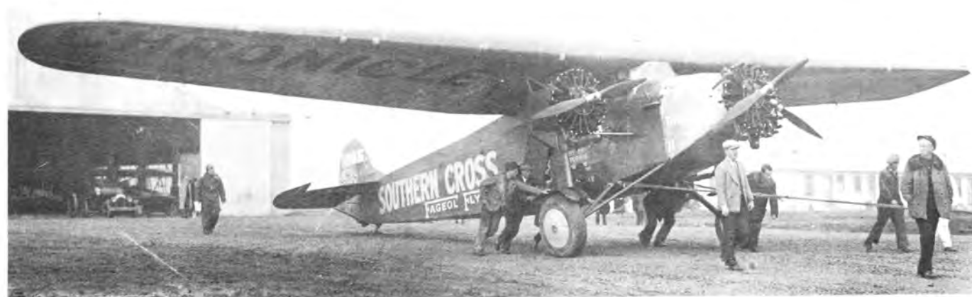
The second Fokker Trimotor, originally built for George Wilkins and fitted with a 71-foot wing, shown as SOUTHERN CROSS, FAGEOL FLYER and SPIRIT OF CALIFORNIA (all at once!) prior to takeoff for first endurance flight attempt at San Francisco. Pilot Kingsford-Smith pulling at the left wheel, copilot Lt George Pond walking behind tail. Original small rudder modified after this flight, wing painted gold and fuselage blue. (Bowers Collection)
