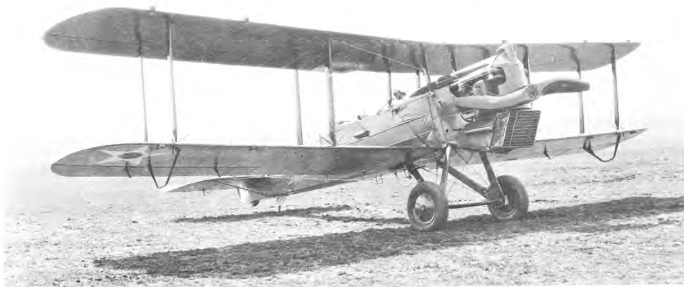
One of the ten DH-4M2S's fitted with supercharged engine. Compare the nose contours and radiator location with the standard DH-4 nose of the XC0-8 modification at the bottom of the page. (McCook Field Photo 30449)
