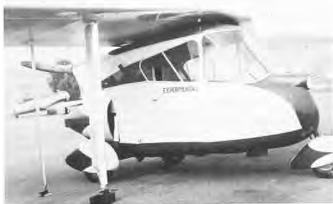
Aerobile's one piece wing had struts that could be angled down and used to raise the wing. (Paul Matt)
