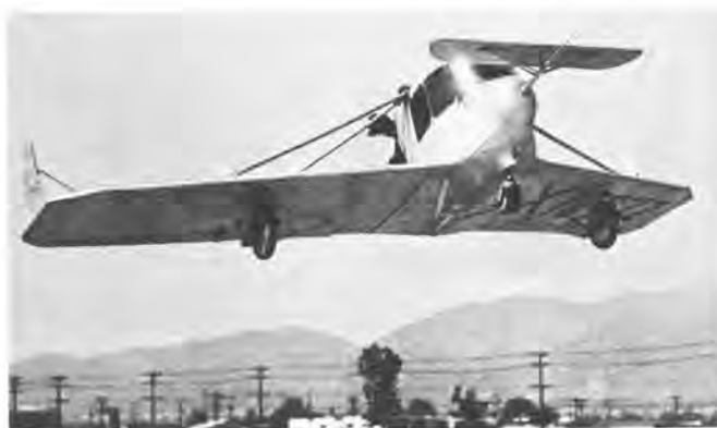
"Whatsit" in late 1932 with new wing and fins, Canard surface and main gear shock absorbers. (Paul Matt)
