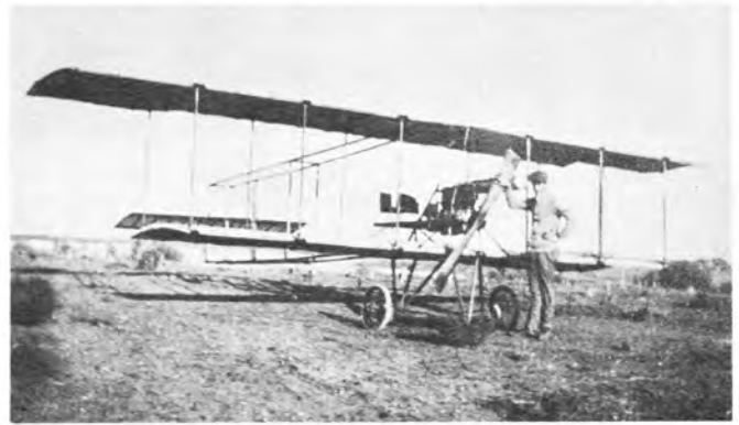
The "Tractor" at North Island, 1912, with Waldo by the propeller. Engine was 20 hp Cameron. (Paul Matt)
