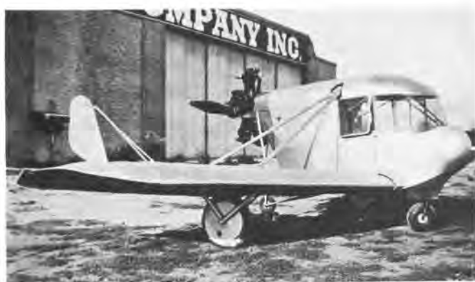
The "Whatsit" in original configuration with small fins wings swept back 15° and extra tail wheel. (Paul Matt)
