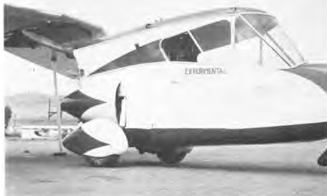
With struts jacked up and wing raised, the automobile pod of the Aerobile could be driven away. (Paul Matt)
