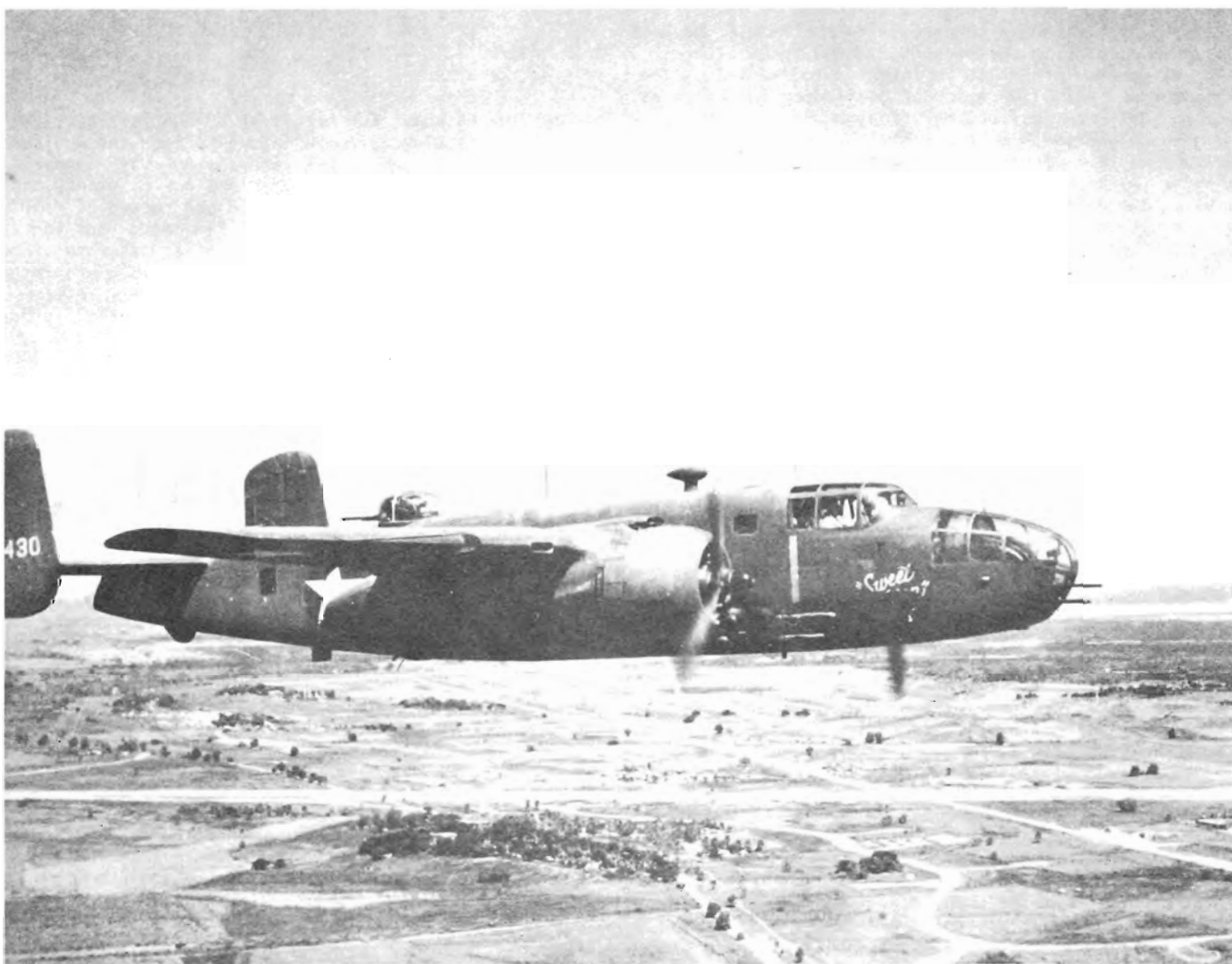
A North American B-25C, "Sweet Eva", 42-53430, of the 70th Squadron over Fiji during 1943. Field-mounted package guns are on sides of fuselage, a feature standardized on later production models of the B-25 Mitchell.
