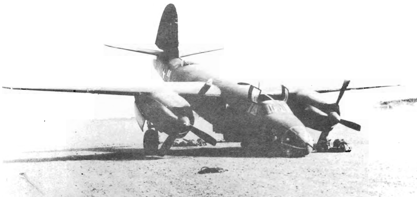
"The Peace Terms", 41-17579, flown by Lt Sherlock in early 1943. Weak nose gear struts were a common early fault.
