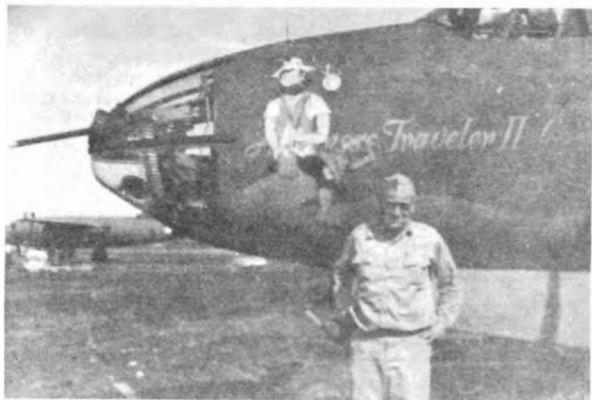
"Arkansas Traveler II" with steel bands added to the nose in the field to help support .50 cal. nose gun.
