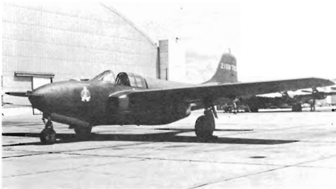
The "Mystic Mistress", two-seated YP-59A, 42-108783, in black paint finish. This airplane was the "Mother" used to control the drone aircraft. (Esposito Collection)
