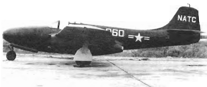
BuNo 63960 at Patuxent River in July 1947 with redesigned vertical tail surfaces and ventral fin. (W. Larkins)
