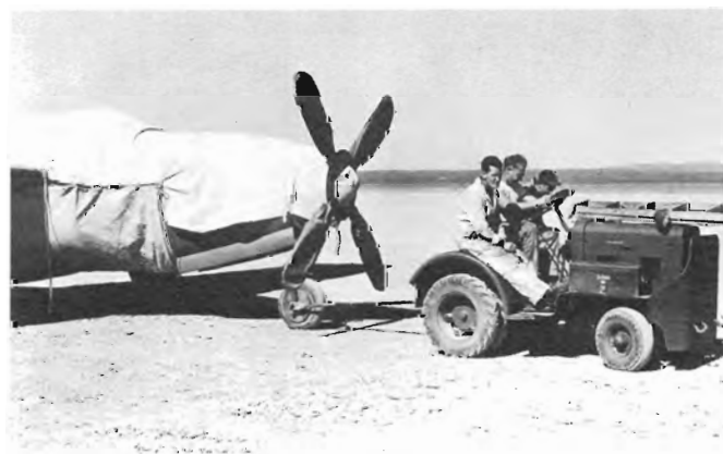
Second XP-59A, 27-2, with canvas covers and dummy propeller used while the airplane was being moved from one site to another. (Bell Aerosystems)
