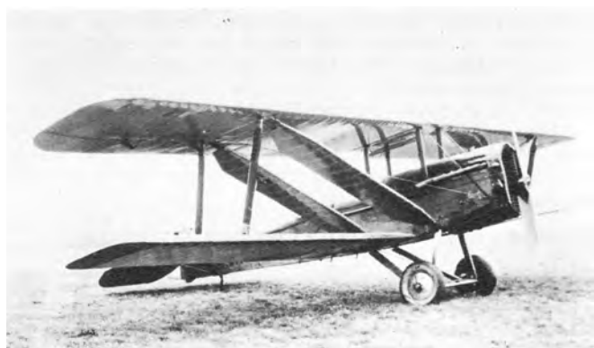
Top: Giuseppe M. Bellanca in his first airplane at Hempstead Plains Flying Field, New York 1915. (Photo - William H. Sheahan of Philadelphia, Penna) Below: Two photos of one of the de Havilland DH-4 aircraft modified with Lifting Struts by G. M. Bellanca—mentioned in Bellanca article in Vol 10, No 1, p 42. (Photos - James J. Sloan)
