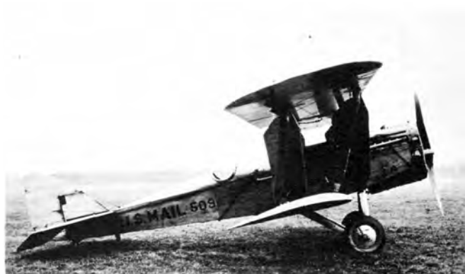
Top: Giuseppe M. Bellanca in his first airplane at Hempstead Plains Flying Field, New York 1915. (Photo - William H. Sheahan of Philadelphia, Penna) Below: Two photos of one of the de Havilland DH-4 aircraft modified with Lifting Struts by G. M. Bellanca—mentioned in Bellanca article in Vol 10, No 1, p 42. (Photos - James J. Sloan)
