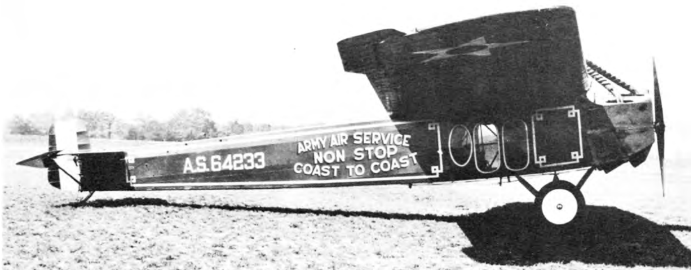
First T-2 after conversion at McCook Field for endurance and long-distance flying. The special lettering for the famous distance flights and the striping are in gold over the standard Army khaki-brown finish. (Photo - McCook 14968)
