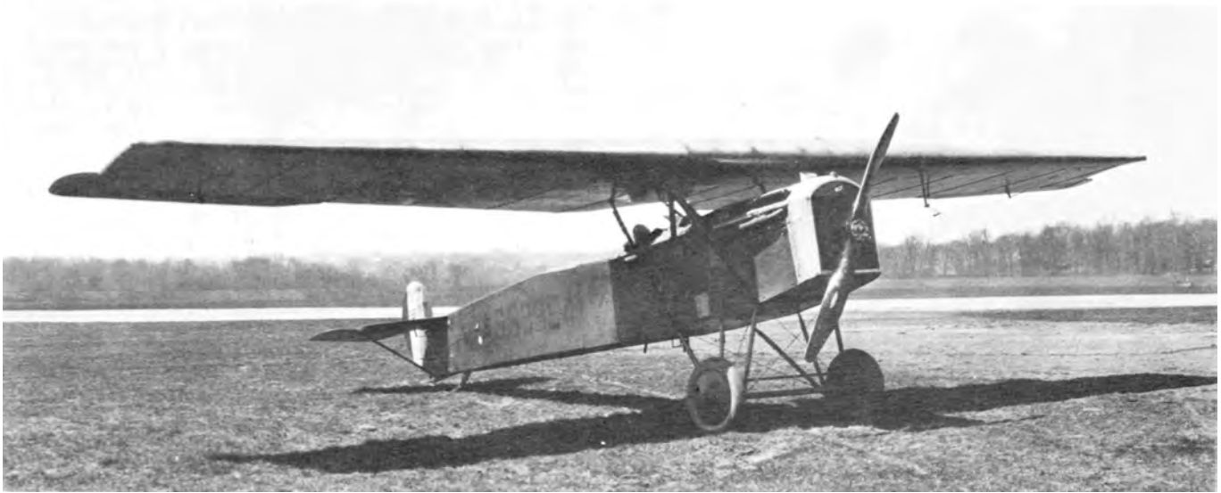
Fokker PW-5, 68554, P-266. Ailerons of the PW-5 extended beyond wing trailing edge, unlike V.40. (McCook Fld 17622)
