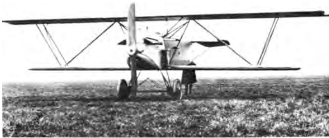
The Fokker D-XII with the Curtiss D-12 engine installed. This was the first attempt by Anthony Fokker to meet the PW-7 requirements. (Photo - McCook Field 13759)
