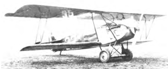
Second CO-4 with round nose radiator, different landing gear and new vertical tail shape. (Photo - McCook Fld)
