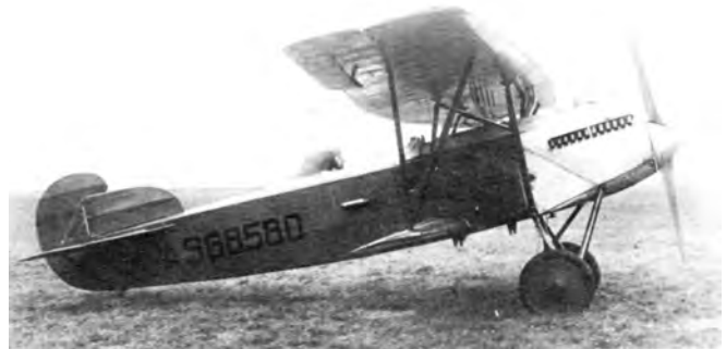
First PW-7 with original tail, headrest and V-struts. Air Service serial number has been applied to the side of the fuselage but there is no insignia. (Fokker)
