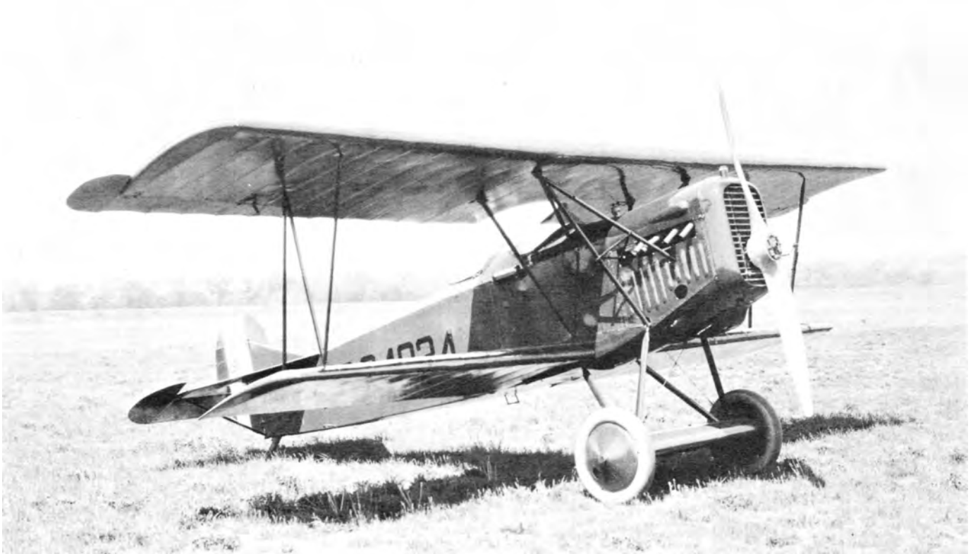
Two-seat D-VII, Army serial 94034, with pilot's seat moved forward and experimental Liberty-8. (McCook Field 17989)
