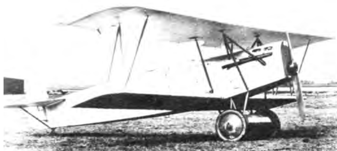
Original form of first Air Service CO-4 (Fokker C-IV), with square nose radiator and axle gas tank. (Fokker)
