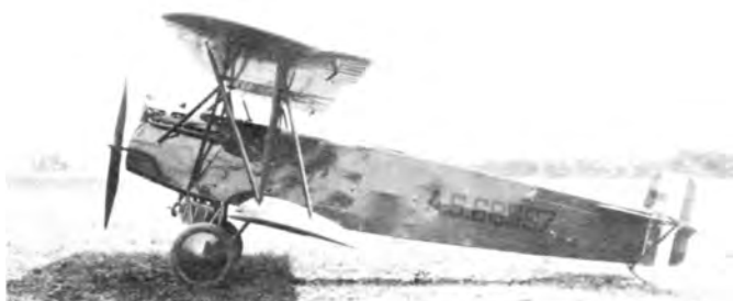
The first CO-4 after change to French Lamblin radiators and elimination of axle gas tank. (McCook Fld 13754)
