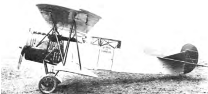
Civilian Fokker C-II, a modified C-I with two-seat rear cockpit and a deep oval radiator. (American Fokker 303)
