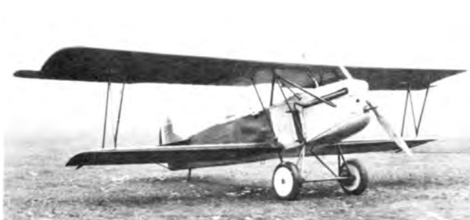
Last of four CO-4A's, 23-1209, delivered with retractable side radiators. (Photo - McCook Field 20247)
