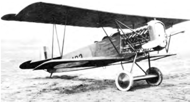
D-VII fitted with the 300 hp Packard 1A-1237 engine was one of at least four so modified at McCook Field. Aircraft is serial 8403 with no P-number. (McCook Field)
