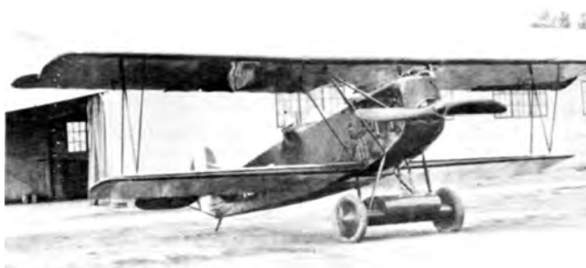
Photographed at Quantico, Virginia this U. S. Navy Fokker C-I shows the landing gear gas tank between wheels and its D-VII radiator. (Photo - U. S. Navy 185553)
