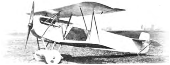
D-IX during its early tests in Holland with the landing gear gas tank installed between the wheels. (Fokker)
