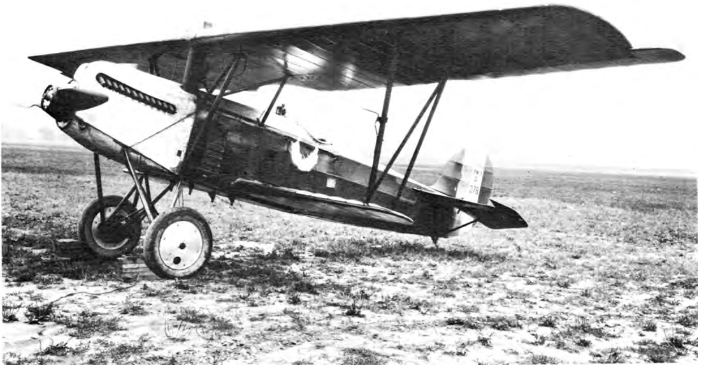
Third PW-7 with revised tail shape used on all three. No. 2 also had fabric covered wings and N-struts. (ScottFld)
