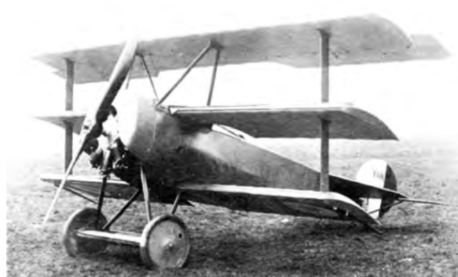
Captured Fokker DR-I tested by the French after being fitted with a 110 hp Le Rhone rotary engine and Nieuport 21 cowl. (Photo - McCook Field 33393)
