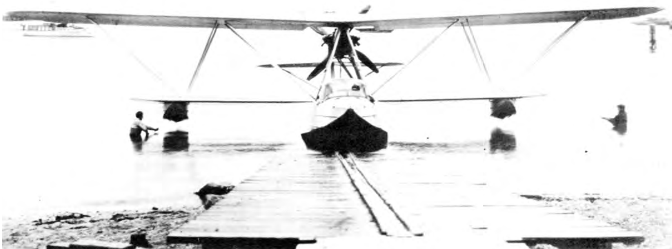
Metal-hulled Fokker B-III was civil version of the open cockpit model built for the Dutch Navy. (Amer. Fokker 555)
