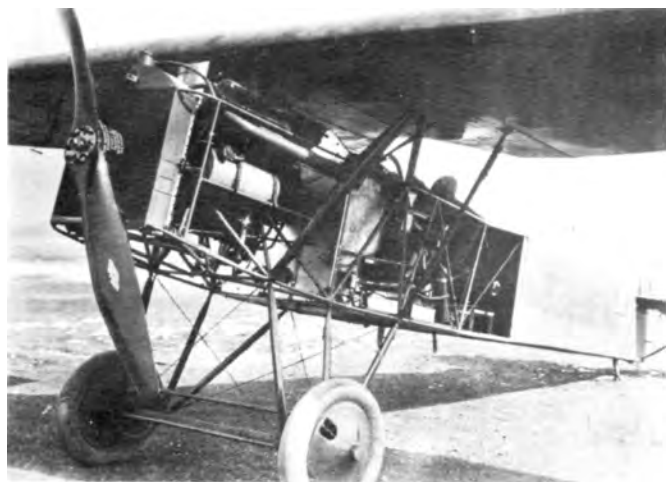
Third from last Fokker PW-5, serial 68554, with engine and cockpit armor removed. (Photo - McCook Fld 16859)
