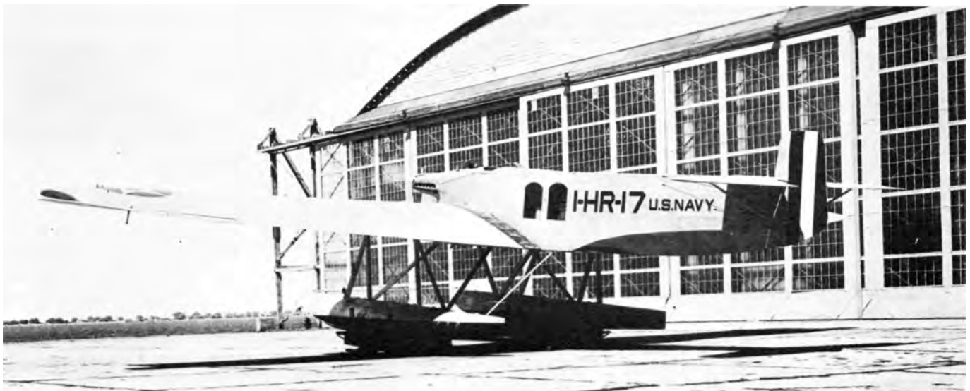
Fokker T-II used by the U. S. Navy as the FT-1. Letters "HR" on fuselage indicate Hampton Roads. (USNavy 651096)
