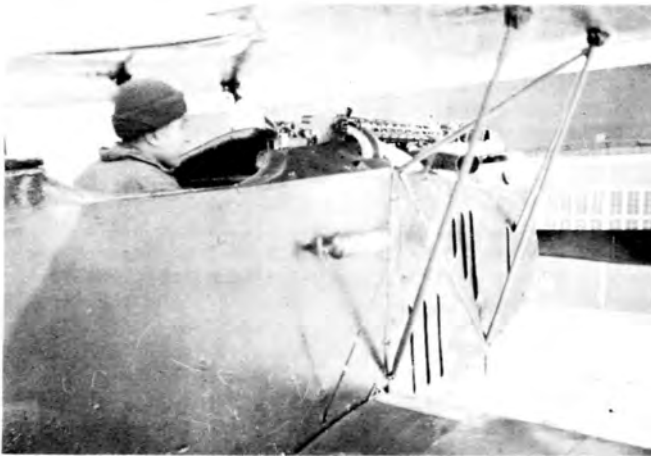
U. S. Army Fokker C-I with German L.M.G. 08/15 "Spandau" machine gun installation. (Photo - McCook Field 11796)
