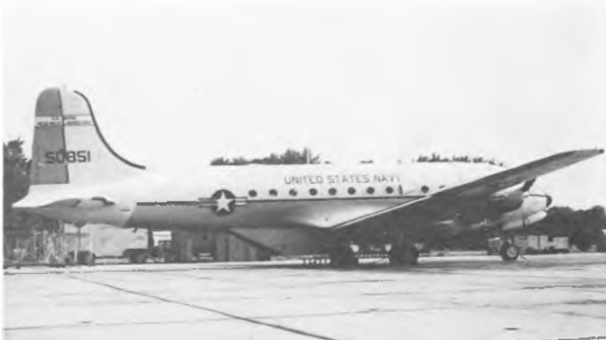
Douglas C-54P, BuNo 50851, with underbelly searchlight, orange under fuselage, fin, elevator and outer wings.
