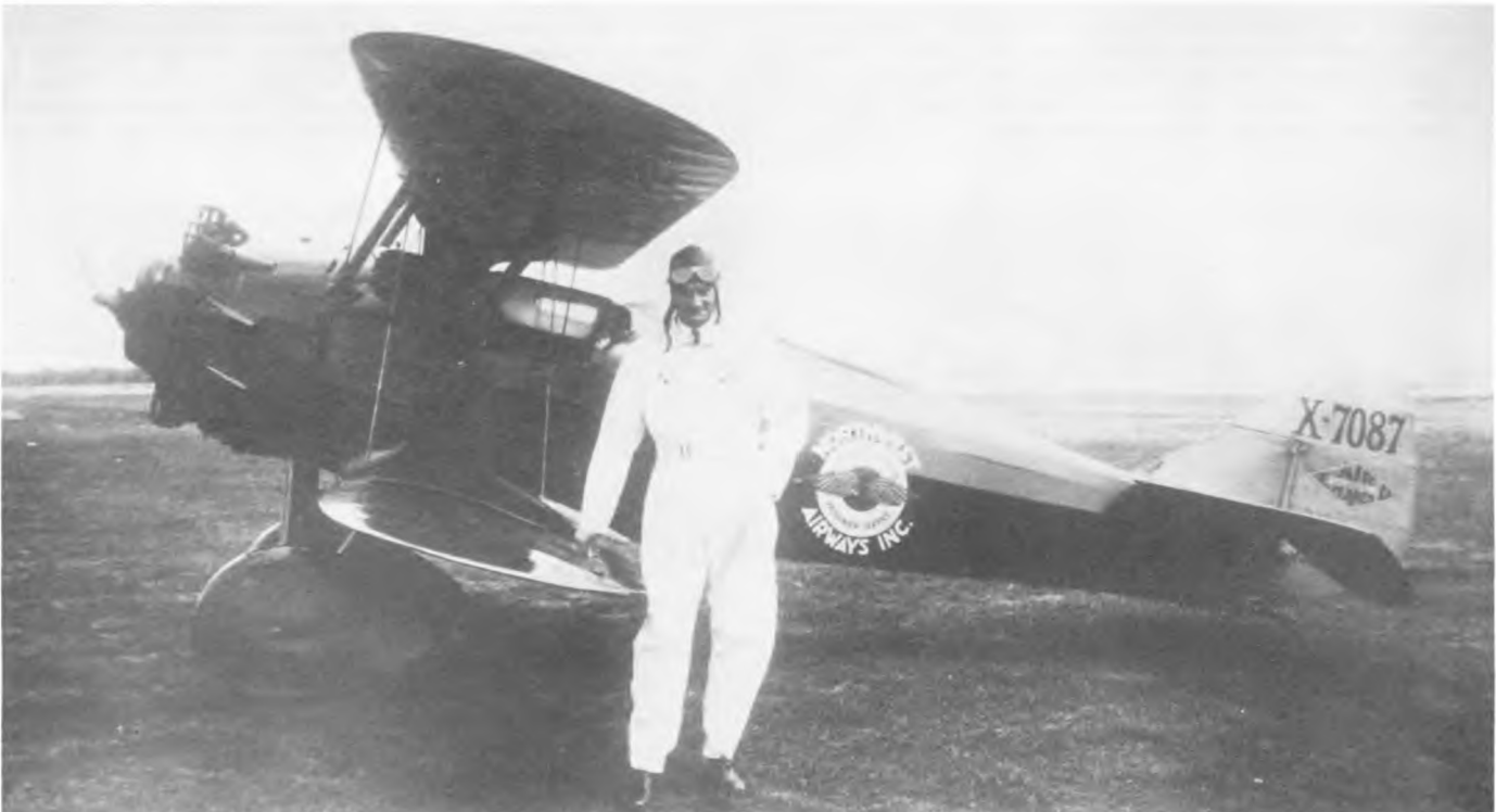
Speed Holman and Laird LCR, X 7087, which later carried racing number "40". Wheel pants and streamlined exhaust stacks have been fitted and plexiglass hatch over the front cockpit is visible. (Photo - Northwest Airlines)
