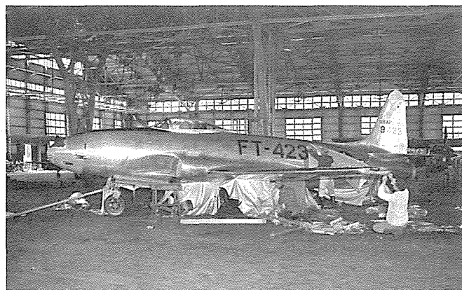
Protective coating is stripped from F-80C in the Corrosion Control hangar at Kisarazu. (Photo - A. Dolim)
