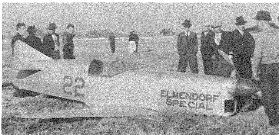
#22, "Elmendorf Special" (Keith Rider R-5), license NX 264Y, Menasco B6S, cream and black. Entrant-Pilot: Dave Elmendorf. Similar to the R-4, Schoenfeld Special, #22 had two foot more span and was some 80 lbs. heavier. The only Keith Rider known to have been built by someone other than Rider. First appeared at the '36 Nationals, did not race at all in 1937 and, after the accident here, was sold to the Marcoux-Bromberg combine, rebuilt, modified and flown as the "Jackrabbit" by Earl Ortman. It is now owned by Jim Garvin, Walnut Creek, California. (Photo - William T. Larkins)
