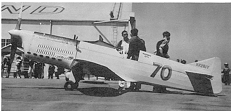
#70, "Firecracker", Schoenfeld Special (modified Keith Rider R-4), license NX 261Y, Menasco C6S4, yellow with maroon letters. Entrant: William Schoenfeld. Pilot: Tony LeVier. Departing from his usual monocoque construction, Rider built the R-4 with a steel tube, fabric covered fuselage entering it in the 1936 Nationals. Schoenfeld bought the plane late in 1936 and hired Rider's crew to rebuild it. He entered it in 1937 Nationals with Gus Gotch as pilot. He then turned it over to LeVier who rebuilt it and came to Oakland. (Photo - William T. Larkins)
