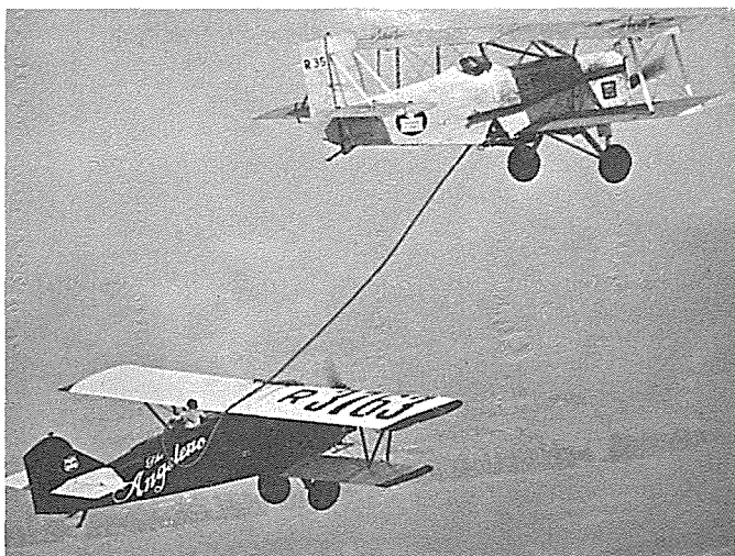
Buhl Airsedan, "The Angeleno", R-3763, taking on gasoline from Curtiss Carrier Pigeon refueling plane, during 1929 endurance flight. (Photo - Piedmonte Coll.)
