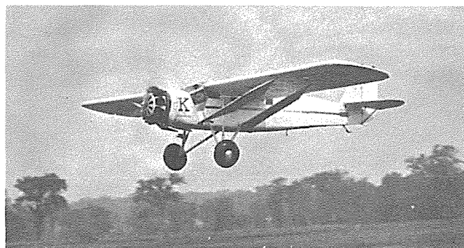
The "K" taking off at the beginning of the first flight attempt to Buenos Aires, 31 May 1930. Aircraft now has balloon type tires and some of the external marking has been altered, including a "K" under the right wing.
