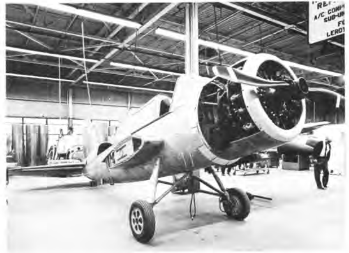
With much of the rehabilitation work done, the OS2U stands at Brookley AFB. Engine, prop, instruments and guns were gone. A main float will be obtained through use of a surplus float from another type. (Edington)
