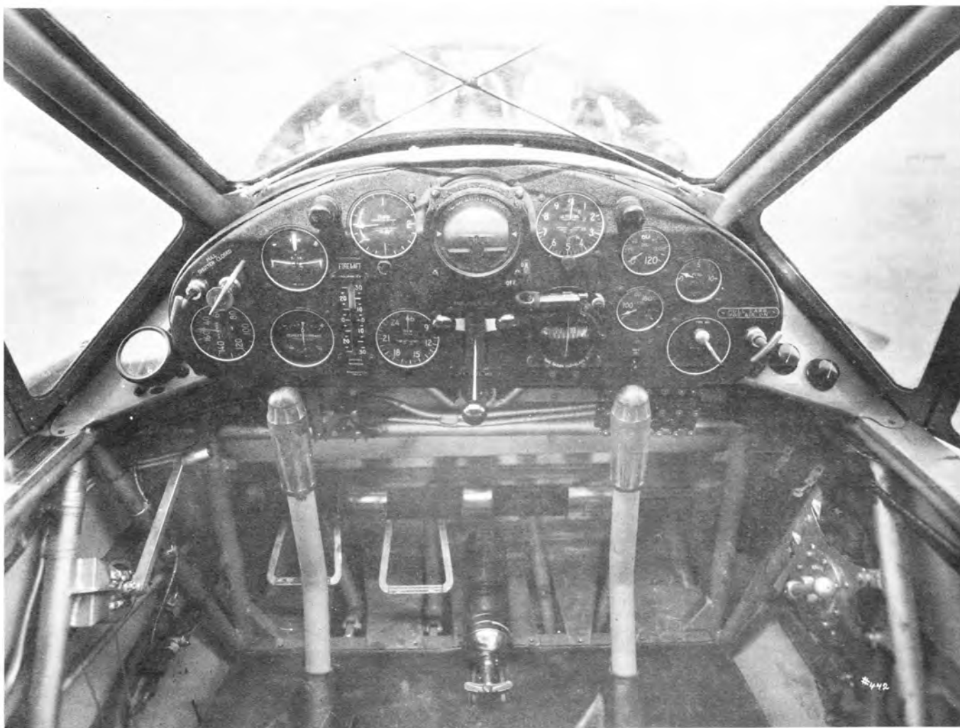
Cockpit interior of the "Liberty" [from 1]: Top row--Turn & Bank Indicator; Rate of Climb Indicator; Sperry Artificial Horizon; Altimeter; Oil Pressure Gauge; and Fuel Pressure Gauge. Bottom row--Air Speed Indicator; Earth Inductor Compass; Rieker Pitch Indicator; Tachometer; Throttle, Mixture and Spark Controls; Daiber Ball Compass; Oil Temperature Indicator; and Ignition Switch. (Photograph - Felipe E. Ezquerro)
