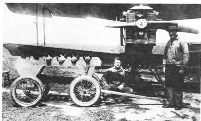
SE-5s at Langley were also used to carry small bombs which were attached to the aircraft beneath the fuselage as seen here, 3 June 1921. (Olmsted Collection)
