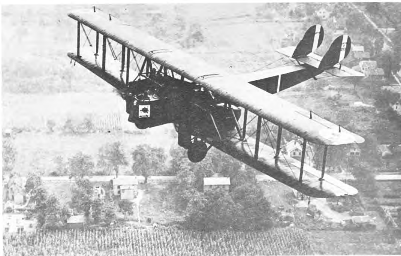
Curtiss NBS-1, serial 68508, of the 20th Bomb Squadron and carrying McCook Field number P 293. Engine radiators are underslung, in the position used with turbo superchargers, though they are not installed here. (Olmsted Coll.)
