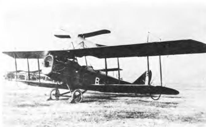
Curtiss JNS Jenny of the 50th Observation Squadron with G-1 target glider fitted to its upper wings during the early part of 1925. (Photo - John Brogan)
