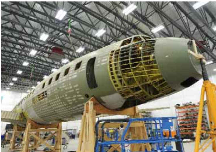
Above: Cabin area looking forward toward cockpit. The plans are to reverse the freight door conversion back to the original passenger entry.
