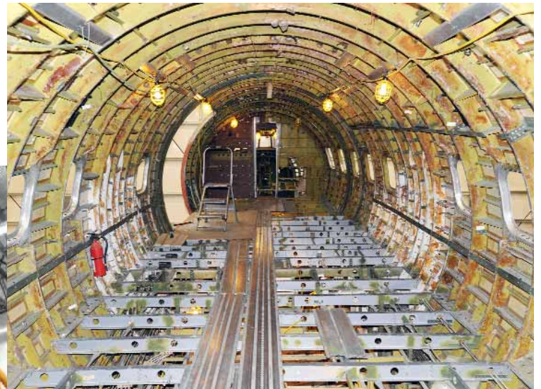
Above: Cabin area looking forward toward cockpit. The plans are to reverse the freight door conversion back to the original passenger entry.
