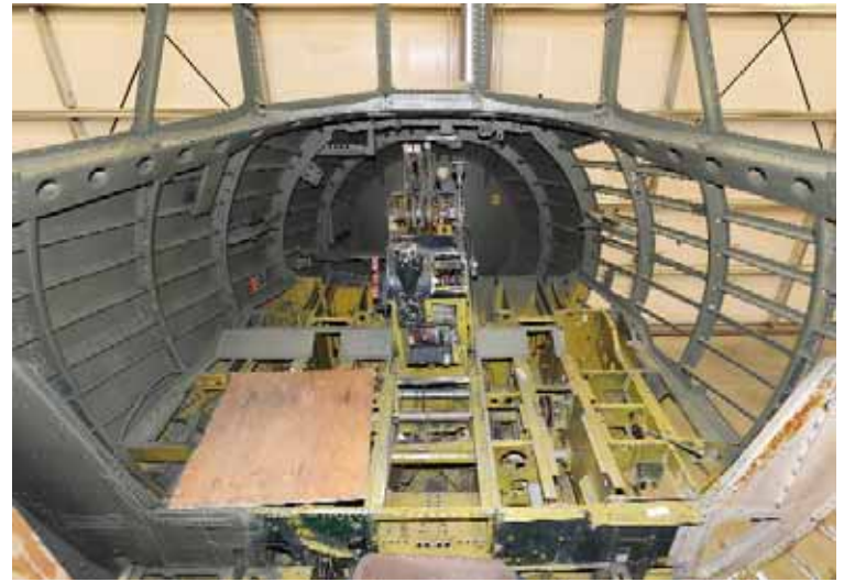
Cockpit area stripped down to the basic airframe.
