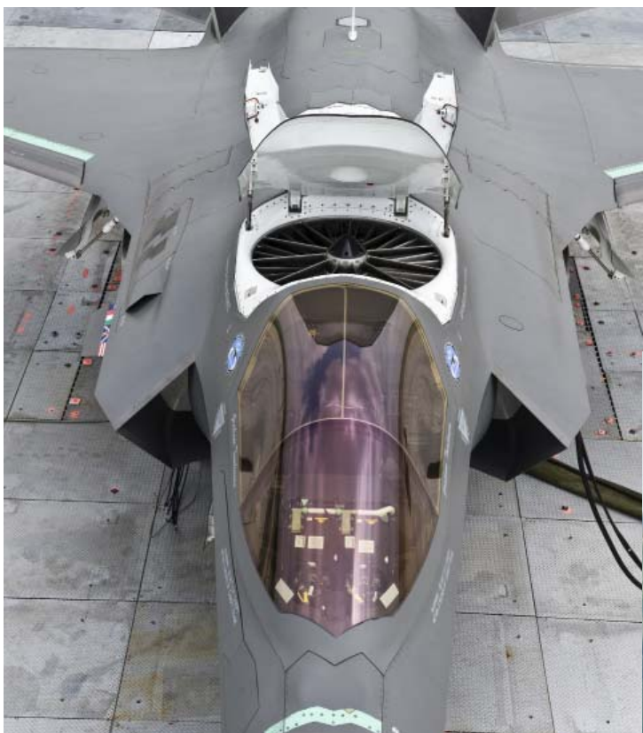
View of the forward lift fan and intakes of the F-35B. (Lockheed Martin photo)
