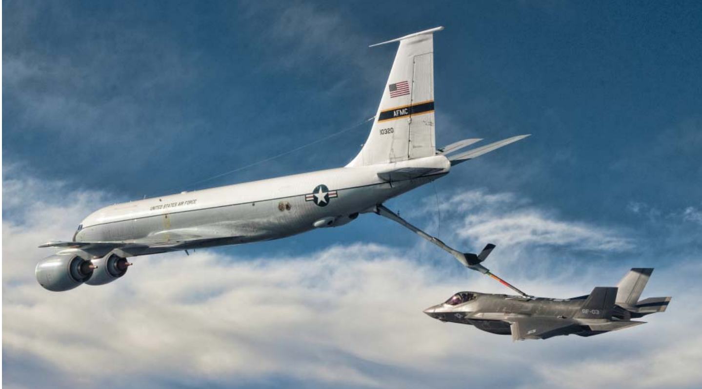
First inflight refueling hook-up with F-35A, AF-03. (Lockheed Martin photo)
