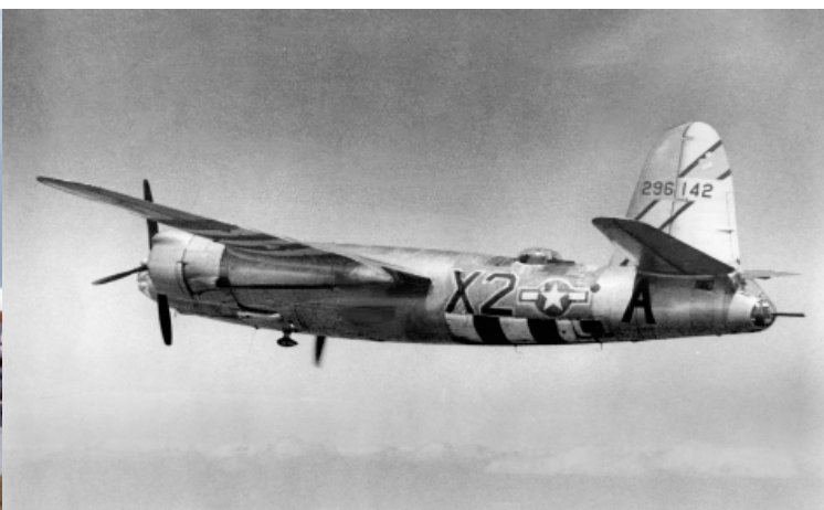
Martin B-26B-55 Marauder, 42-96142, in D-Day markings with the left engine feathered and oil streaming from the exhaust. (Martin photo from the AAHS photo archives, AAHS-P010109)
