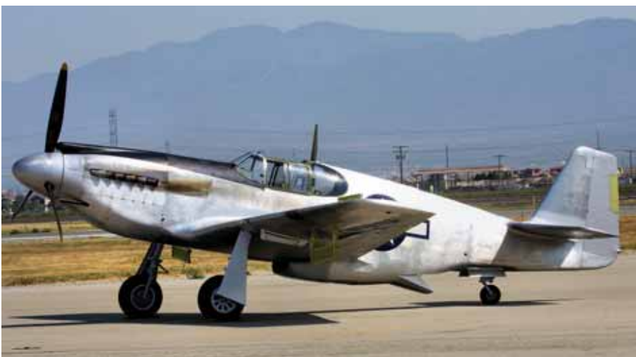
A rare airworthy A-36, 42-83731, NL251A, attended the air show. Note the dive brakes deployed in front of the flaps above and below the wing. (All photos by Chuck Stewart)
