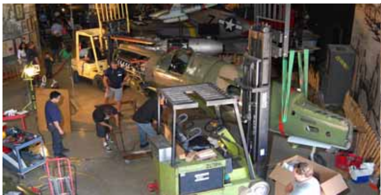
Fighter Rebuilders’ John Hinton (top) and Cory O’Bryan (lower left), and Don Russell of the San Diego Air and Space Museum staff prepare the support cradle to receive P-40’s fuselage and engine. (Photo by author)
