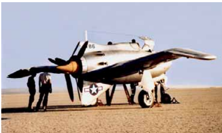
Northrop XP-56, 41-786, at Muroc (Edwards) AFB in October 1943 showing fin modifications. (Northrop photo from the Gerald Balzer collection, AAHS-P005682)
