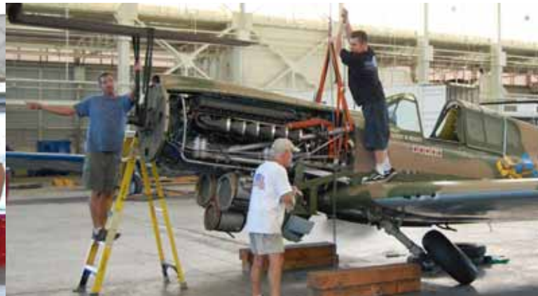
The airplane is being raised and the gear extended. Shortly afterward, the airplane was set on its wheels and the overhead suspension released. (Photo by the author)
