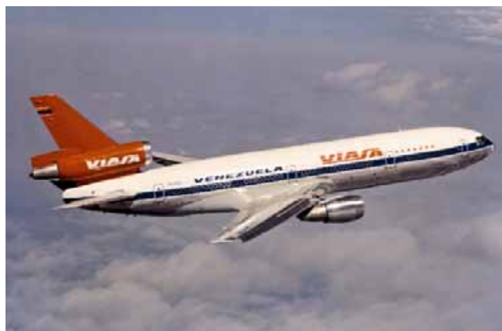
Viata Airlines McDonnell-Douglas DC-10-30, YV-137C, s/n 46982, in slow flight with leading edge flaps deployed. (Photo from the Kase Dekker collection, AAHS_P004510)
