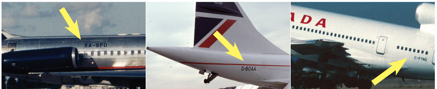
Here are a couple examples of different country registrations. From left to right an Aeromexico MD-80, XA-SFO, British Airways Concorde, G-BOAA, and an Air Canada L-1011, C-FTNG.
