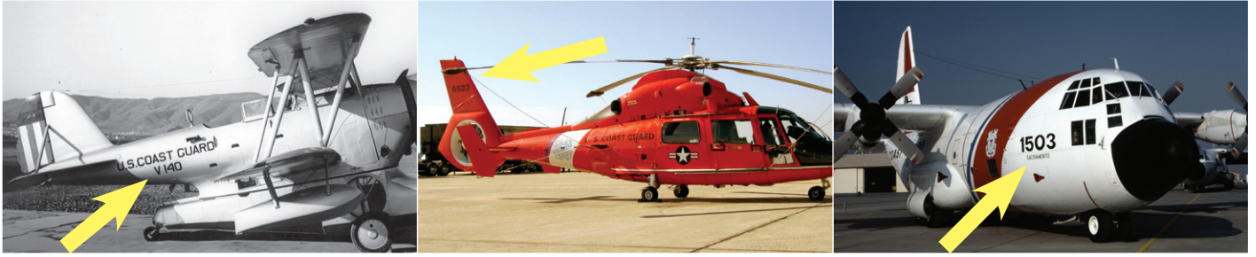
Here we see examples of three styles of USCG registration numbers. Left is a 1930s era V- number, center a four digit number which represents an aircraft within a block of id's, and right a registration number prefixed by a "1" followed by the serial number. Confusing to say the least, but because there are not a lot of USCG aircraft, easily to quickly look up in the reference given.
