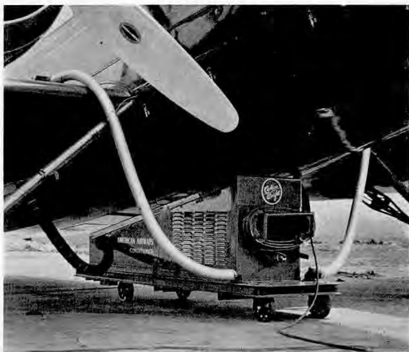
AIR-CONDITIONING A SLEEPER PLANE
