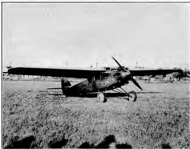
"Cessna" Cabin Monoplane. Engine, Wright "Whirlwind."
