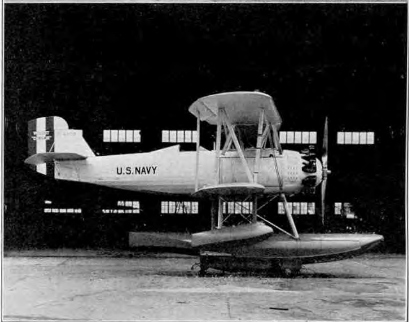
(Top) The Vought "Corsair" Planes used by Asst. Secy. of the Navy Warner, and Admiral Wm. A. Moffett, Chief of Bureau of Aeronautics, Navy Dept. for inspection trips. (Bottom) The Vought "Corsair" Seaplane (all-metal float gear). Both types equipped with "Wasp" engine.
