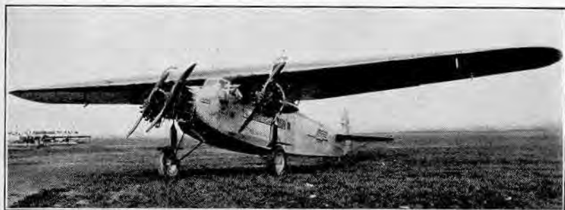
Pan-American Airways, Inc. Fokker "Tri-motor." Engines, "Whirlwind."
