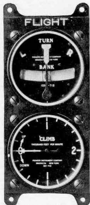
Pioneer Flight Indicator. Turn and Bank Indicator combined with Climb Indicator.
