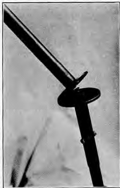
The Alexander Aircraft Company Spring Safety Stick designed to prevent accidents in training due to a student "freezing" to the controls.
