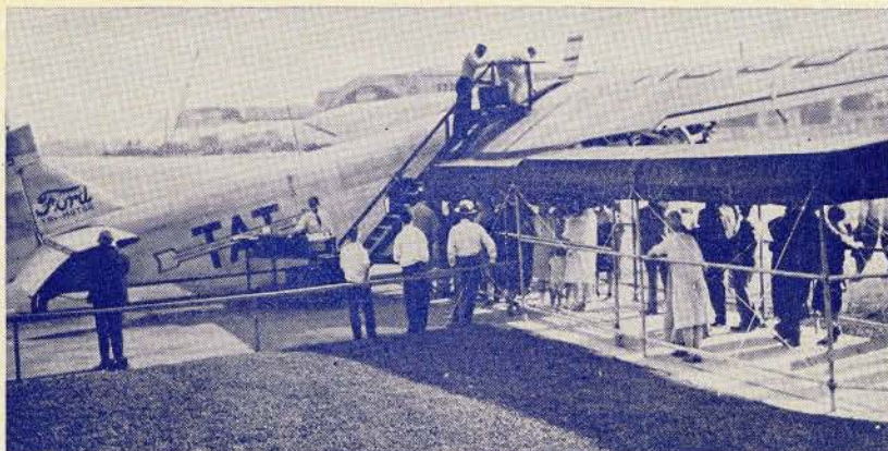
T A T station attendants putting passengers' baggage into the wing of the transport plane, at Port Columbus, Ohio.
