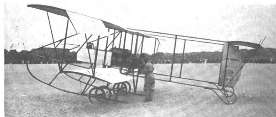
An improved type of biplane turned out by the English Bristol Co. Note the skid arrangement running up to the front elevator, the cabin for the pilot and the single tail plane.
