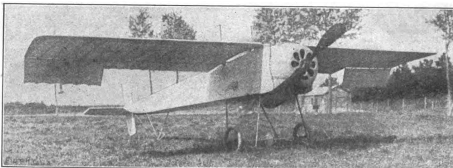
Although the name of Farman is inseparably associated with biplanes, Mr. Henry Farman has for some time past successfully experimented with a monoplane of his own design. We are now able to give the photograph of this machine, perhaps the most striking feature of the external appearance of the machine is the neat stamped-out casing that encloses the 50 H. P. Gnome Rotary air-cooled engine. Also, as may be observed, the entire rectangular body is covered with surfacing material.
