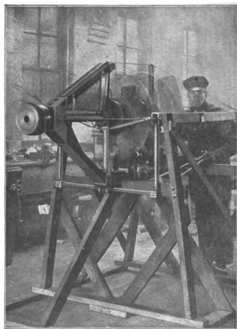
Motor Revolving at 1200 R. P. M.—Nothing Visible of the Propeller but the Hub—Note the Total Lack of Vibrations.
