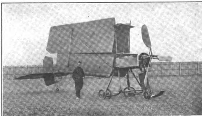
THE BREGUET AEROPLANE WITH WINGS FOLDED FOR TRANSPORTATION OR STORAGE IN SMALL PLACES.
