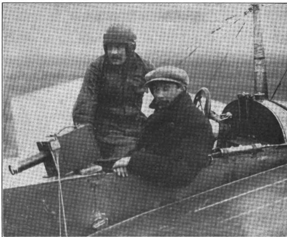
A VIEW SHOWING THE SEATING ARRANGEMENTS OF THE 100 H. P. DEPERDUSSIN MONOPLANE AND KINETOGRAPH IN POSITION READY TO TAKE PICTURES.
