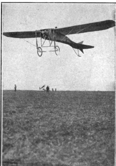
THE LATEST SINGLE-SEATER BLÉRIOT. NOTE THE TAPERING FRAME, FLAT TAIL AND TRIANGLE-SHAPED RUDDERS.
