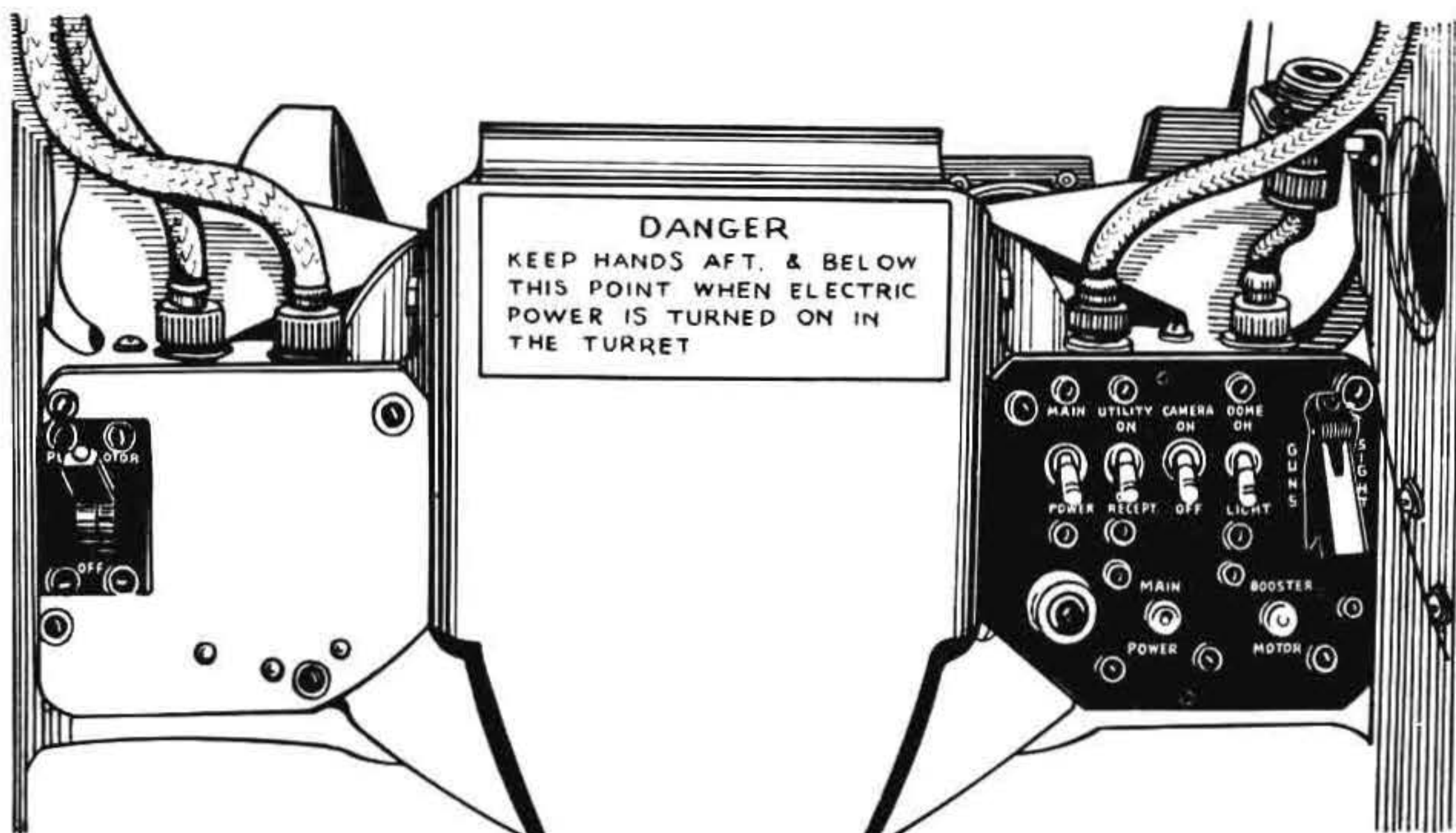
Figure 61 — Turret Control Panels—250CH-1 and 250CH-2
